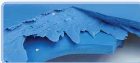
However, when stretching the material and under certain conditions of pressure, temperature and speed, the polymer molecules are aligned in the same direction as the stretching, resulting in a laminar structure.
