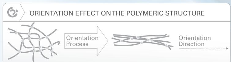
Molecular orientation process modifies the PVC structure by giving the polymers molecules a specific orientation.
