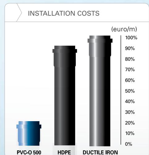
"Based on DN200-250 mm PN16 installation in Europe"
