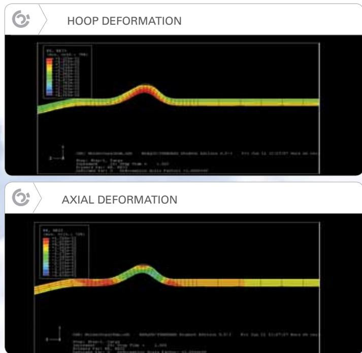
FEM simulation of a PVC-O pipe behaviour with axial and hoop orientation
