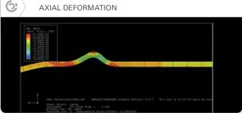
FEM simulation of a PVC-O pipe behaviour with axial and hoop orientation
