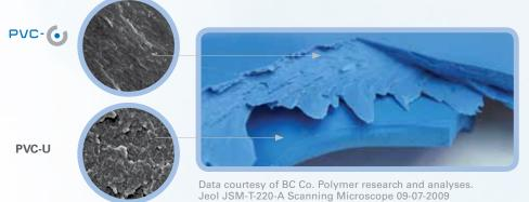
However, when stretching the material and under certain conditions of pressure, temperature and speed, the polymer molecules are aligned in the same direction as the stretching, resulting in a laminar structure.
