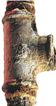
External corrosion - Steel
